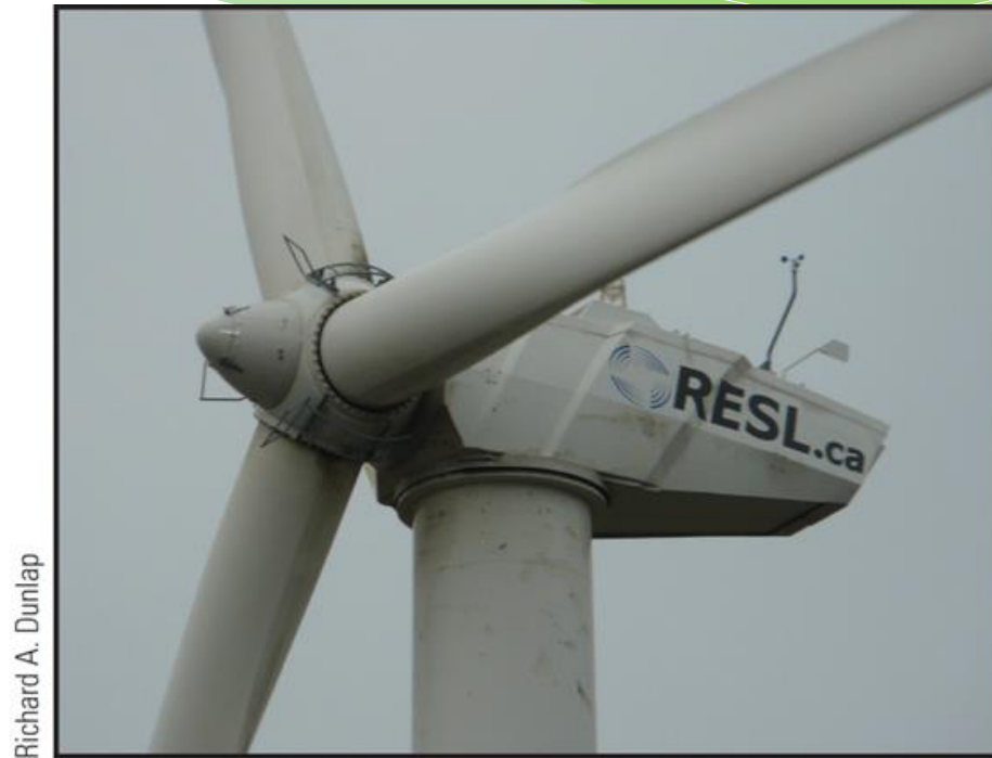
Figure 10.8: Nacelle of a 600-kW wind turbine.
